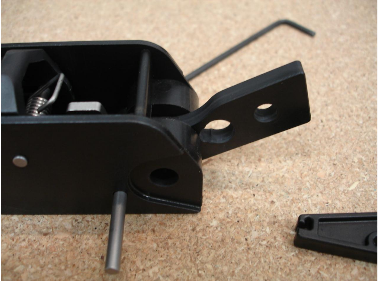
11. Install the new K&M Lightning by tilting it at an angle to get it into the slot.
