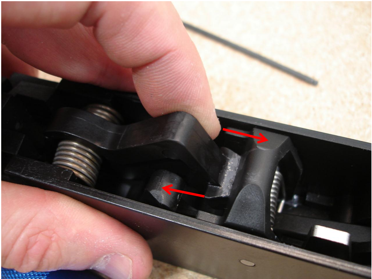
6. Release the hammer by pulling on the sear catch and releasing the trigger catch.
