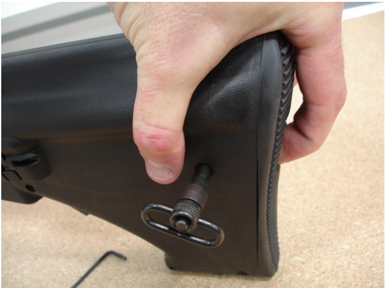
17. Install the sling pin. Now charge the rifle and feel the trigger pull. Change the position of the spring to the desired poundage pull.
